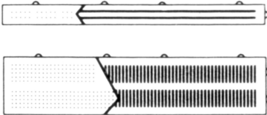
The bus rows, usually 2 on each side, are reserved for positive power and ground. The holes in the center columns are for components. The divider between the columns will be very useful when we start working with ICs (Integrated Circuits). It assures that each pin of the IC has its own column for other parts to be connected to it.
