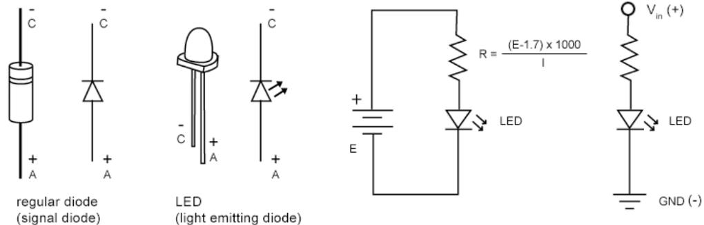
When using a LED in an electronic circuit, use the above formula to determine series resistance in Ohms. Never use a LED without a current limiting resistor in a circuit – in most cases it will explode if you do! R is resistance in Ohms, E is the supply voltage and I is the LED current in milliAmperes (mA). What value for R do we get with our 9/12 VDC power supply and a standard LED (1.7V voltage drop, 20mA current)?
