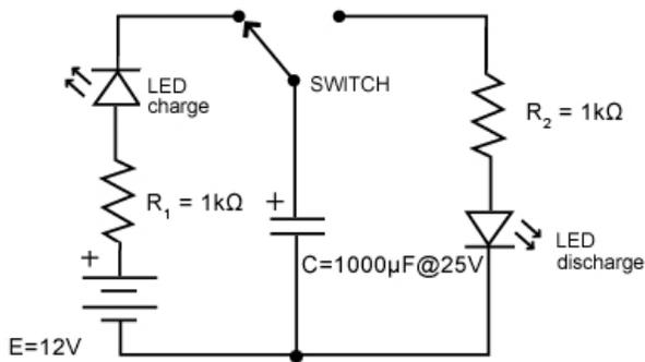
In this experiment, when the switch is moved toward the left side (battery), the capacitor is charged. In this process the LED lights up but gradually fades. When the capacitor is fully charged there is no current flowing through the LED anymore. Now, when we flip the switch over to the right side, the capacitor discharges. This process is again visualized by an LED that gradually dims.
