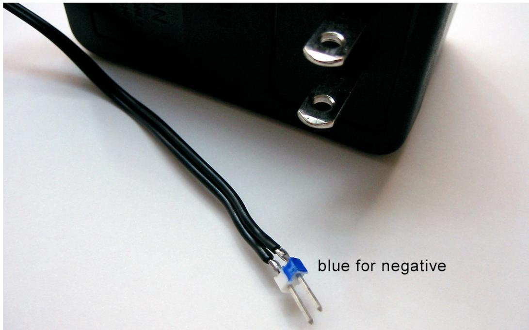
Since direct current only flows in one direction, we have to be able to easily determine the positive and negative side of the power supply. Remember that we assume the conventional current flow from positive to negative when we work with circuits! By convention, positive is always marked with red and negative is always marked with black or blue.
