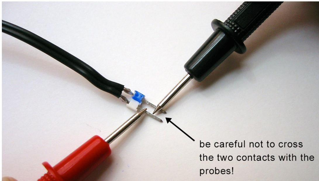
Take a red marker and mark the side of the power supply's header connected to the multimeter's red probe red – this is your positive power supply. Or mark the other side black or red. This is very important. You can blow a circuit easily by applying the voltage in the wrong direction.
