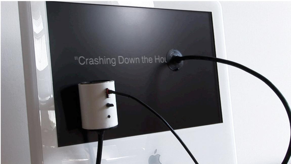
the knob on the elocuter is for volume adjustment, the push button is for calibration purposes (to accommodate brightness differences between different screens).
